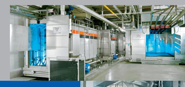
:: The most important component of a good surface is the one you don't see: a good pre-treatment. The materials to be processed are thereby decisive. From steel to aluminium to plastics, Rippert has developed numerous processes for cleaning, degreasing, phosphatisation and etching or for conversion treatment.
